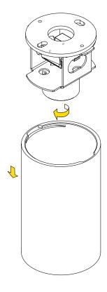
2 Slide plate. Fix and make electrical connection.
